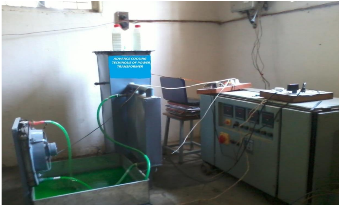
Fig3. Practical working model of cooling system in lab
